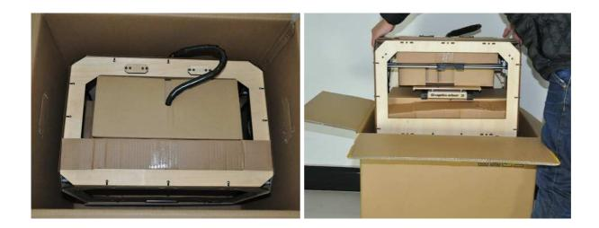
In the packaging underneath your Duplicator 3/4you'll find the **Power Supply** and **cable**, as well as your **USB A to B cable** and **Filament Guide Tube(s)**. Take these out and put them aside.
