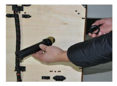
Next, locate your **Filament Guide Tube(s)**. These fit into the tube guide holders at the top of The Duplicator 3's back plate.
