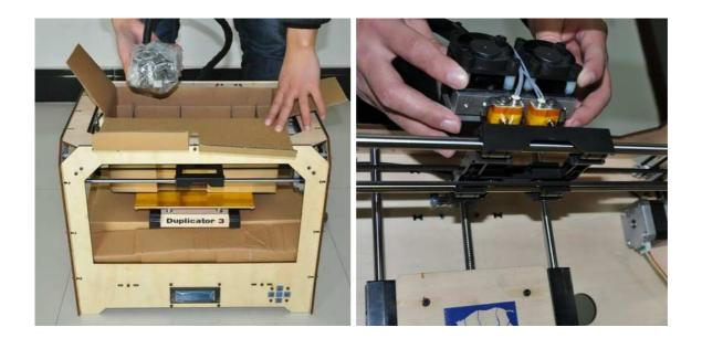
Now you can clear away the cardboard inserts and remove the **Accessory Box** from The Duplicator 3. Be careful of the black plastic **Step extruder MK8+ Mount**.
