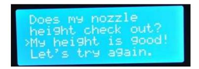
Use the Support card to test the platform height one last time. If the card can move up and down underneath the nozzle, your platform is too low; select "Let's try again." If it can slide around a little bit, you're good to go.
