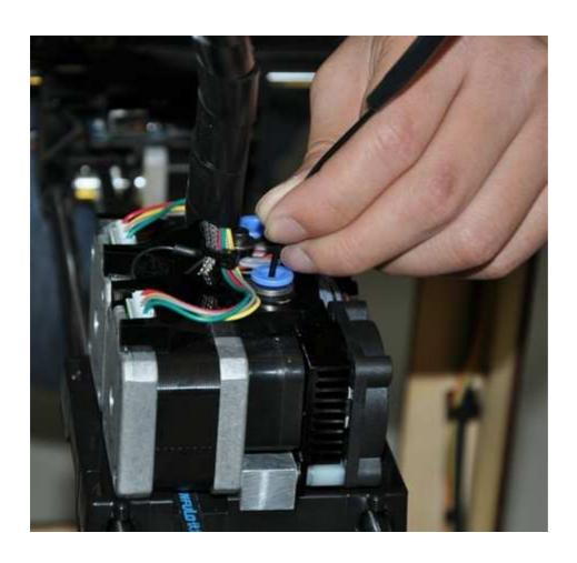
Once the tubes are disconnected, you can go ahead and feed the filament into the guide tubes from the back until you see it come out at the front. 4.4
