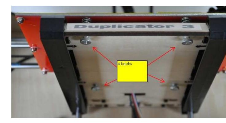
It's very important that you always move two knobs during each step -- if you try to move only one knob at a time, the script can have unexpected results. Also, make sure that you're moving the specific knobs the script is telling you to use.
